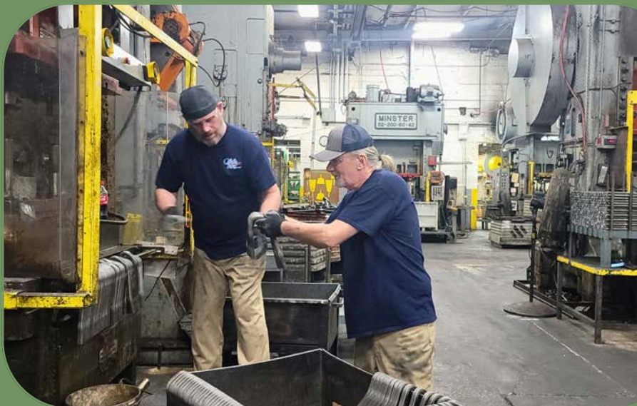
Midwest Fabricating employees pictured cold forming steel into fasteners and custom wire formed rods at the plant located in Amanda, Ohio.
